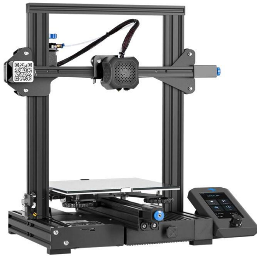
Figure 26. Example of the cartesian manipulator in the form of a 3D printer. Source: [22].
